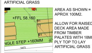
APROX 100M2. ALLOW FOR RAISED DECK AREA MADE FROM TIMBER PALATES WITH 18MM PLY TOP TO LAY ARTIFICIAL GRASS
